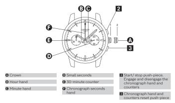
Hour, minute and seconds display. Can be used to time events lasting up to 30 minutes, with a precision of 1/5<sup>th</sup> of a second.
