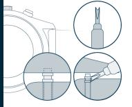
Insert the tool to pull out one side of the bar by pulling the strap against the outside.
