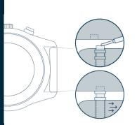
With the tool, press the bar by pushing the strap between the lugs of the watch.
