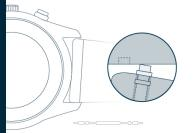
Once the bar is in this position, you can remove the strap.
